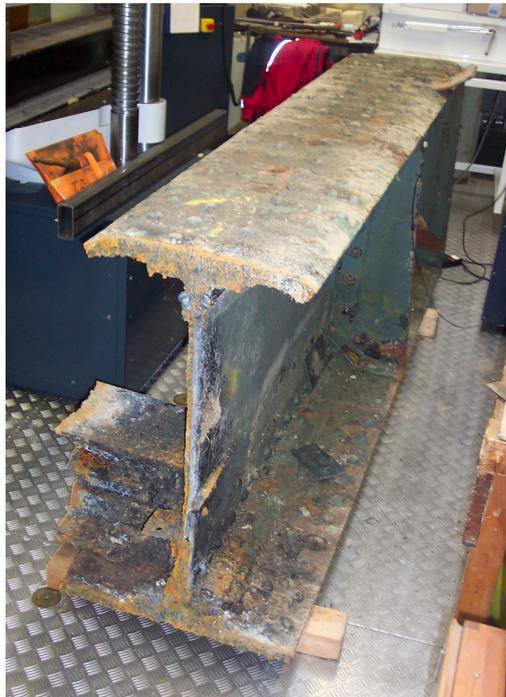
Figure 3.31. A short length of wrought iron I-section beam removed from a railway bridge in Llangammarsh Wells in South Wales.
