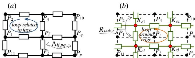
Fig.2. Parts of equivalent magnetic networks: (a) edge - EN and (b) facet - FN
