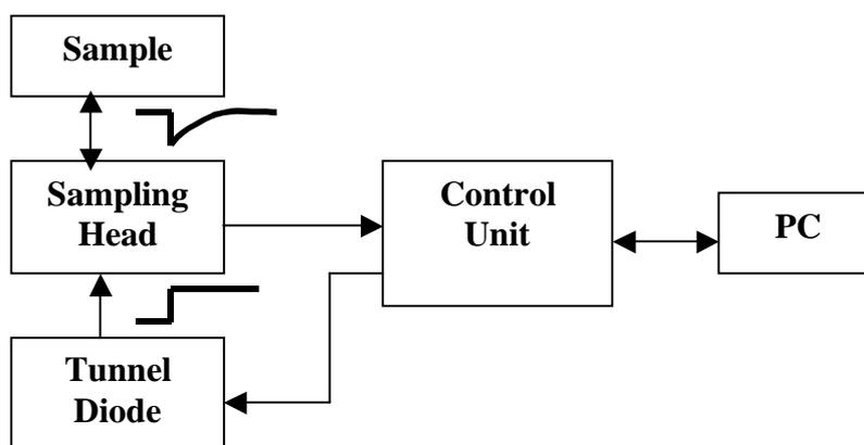
Fig. 2 Schematic diagram of TDS measurement.
