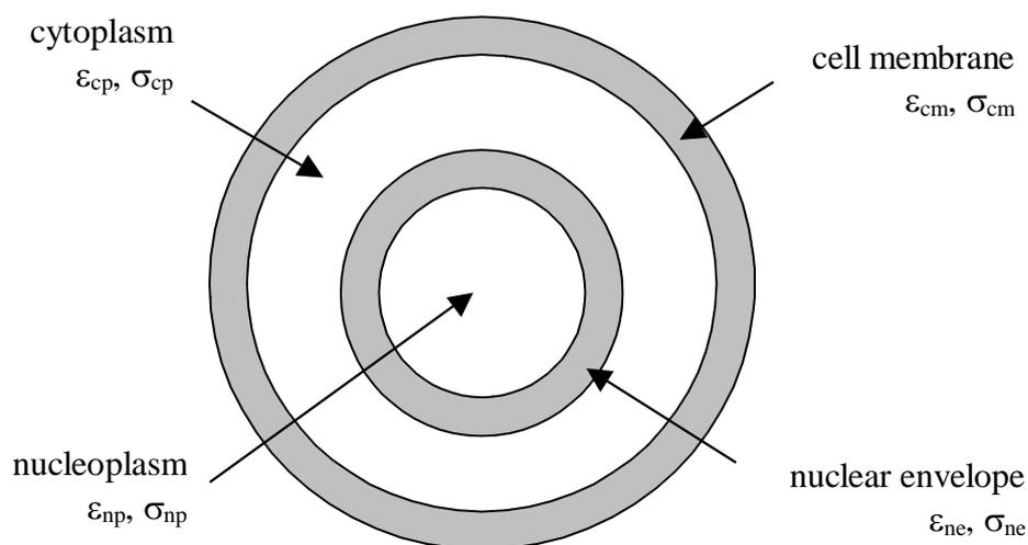
Fig. 1 Schematic picture of the two-shell model of a eukaryotic cell, where  $\epsilon$  and  $\sigma$  represent the permittivity and conductivity, respectively.
